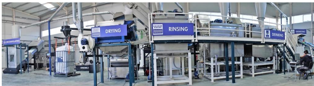
Figure 7: Cadel/Keycycle Deinking Demonstration Plant
