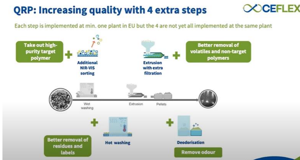
Figure 4: CEFLEX QRP Extra Process Steps for Increased Quality Source: CEFLEX 2021b
